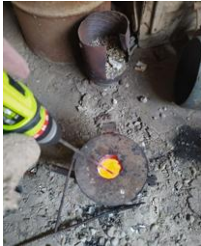
Figure 3. Stir casting process
