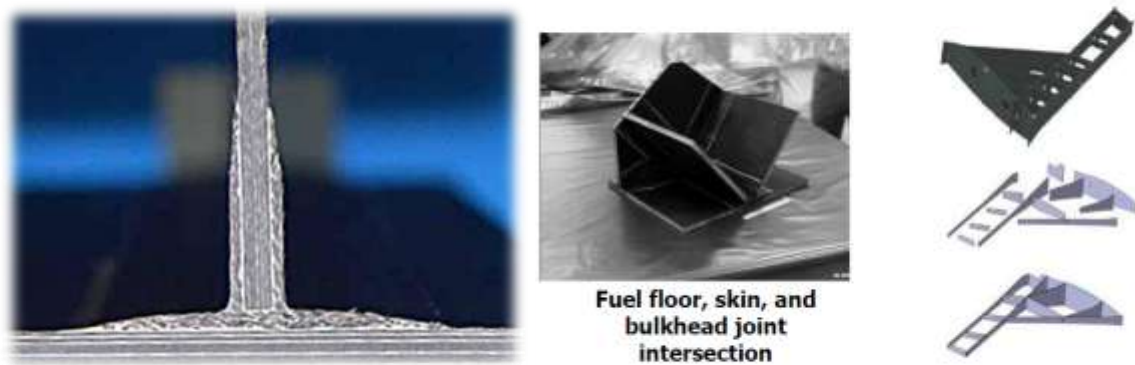
Figure 17 - 3-D Woven and Pi-Preform Joints and Large Integrated Composite Structure [5].
