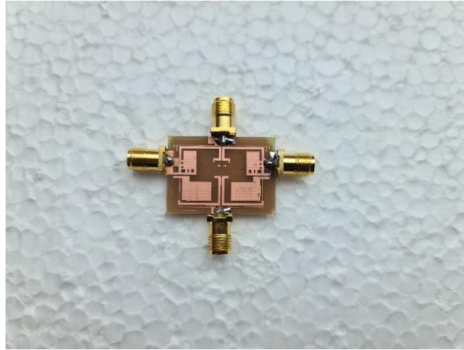
Figure 4. Fabricated coupler using an FR4 substrate as the dielectric.
