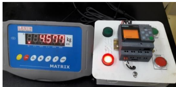
Figure 13. Load cell and PLC screen
