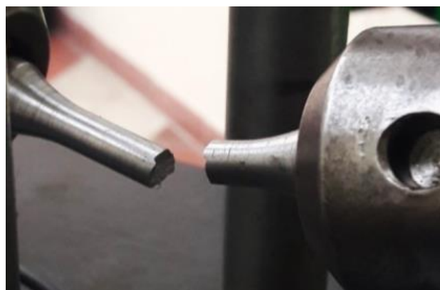
Figure 14. Broken test specimen
