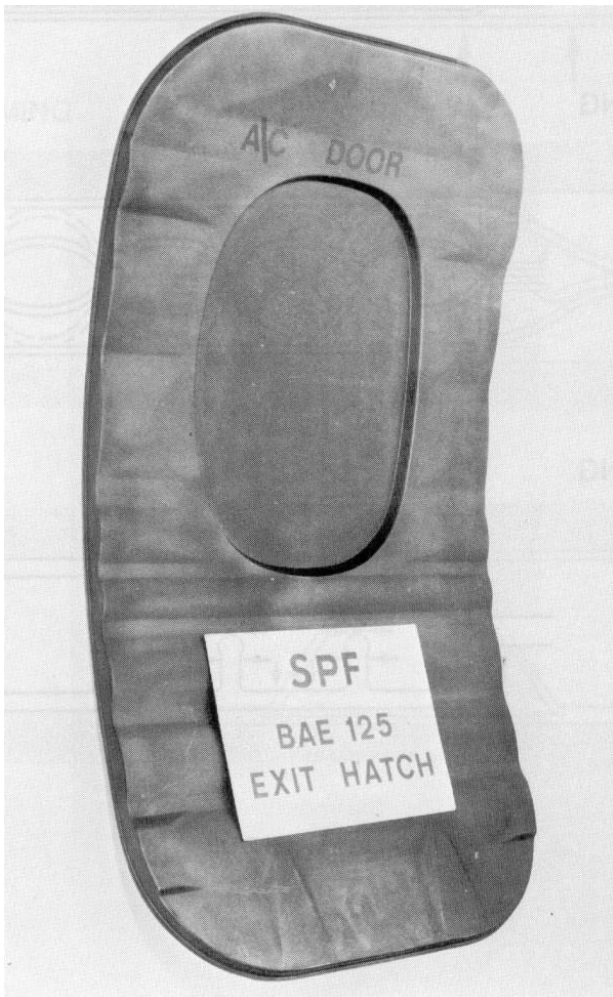
Figure 8: Exit hatch for the BAe 125/800 made of titanium SPF/DFW33
