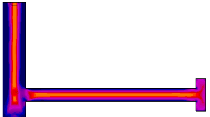
(f) Permanent mould (120°C), cast at 750°C
