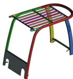
Figure 10. Finite Element Model of Head Guard.
