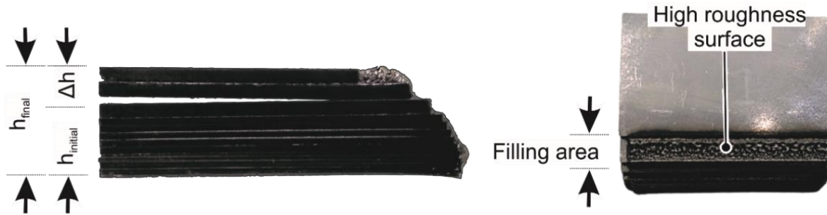
Figure 8. Height deviation \Delta h and welded sample with high roughness for 316L
