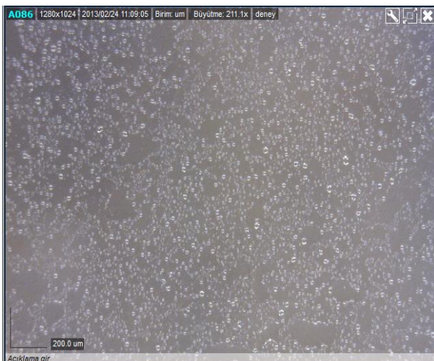
Figure 11 The view of droplets that they are atomized with ultrasonic sound.
