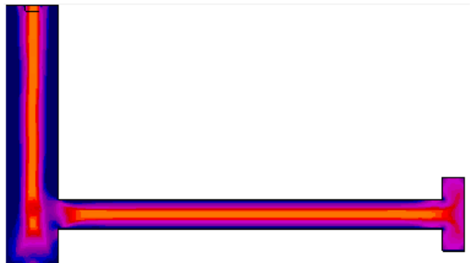
(f) Permanent mould (120°C), cast at 750°C
