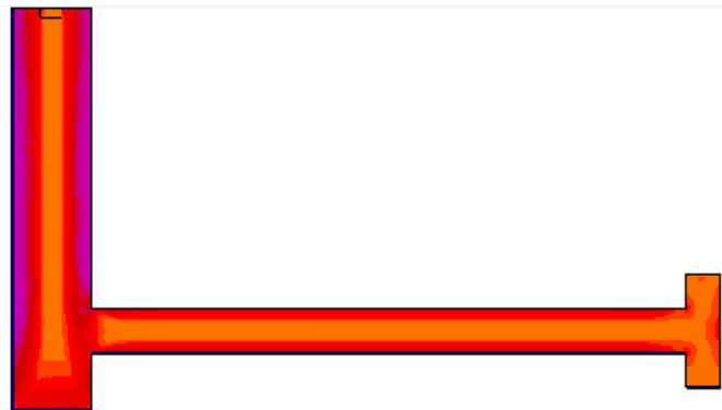
(e) Permanent mould (120°C), cast at 700°C
