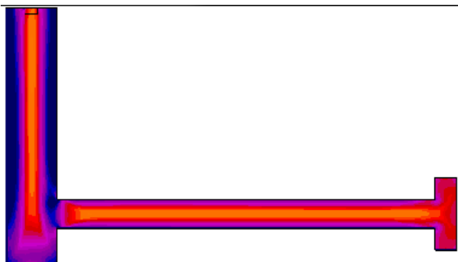
(g) Permanent mould (250°C), cast at 700°C
