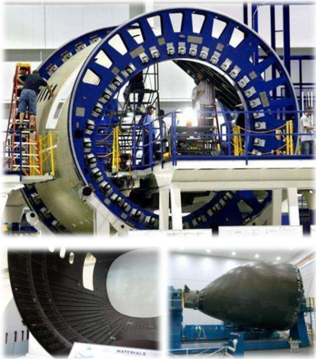
Figure 11 - Composite Material Usage in BOEING 787 Aircraft, Copyright of Boeing Commercial Airplanes, [12].
