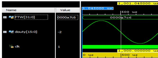
Figure 11. The Generated 1 kHz sine wave (clk =100 MHz)
