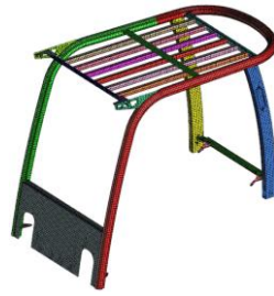
Figure 10. Finite Element Model of Head Guard.
