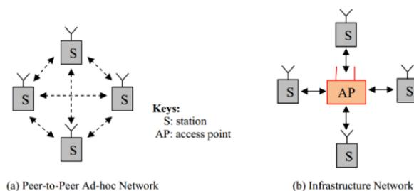
Figure 3. Two types of Wi-Fi are shown as examples [35]
