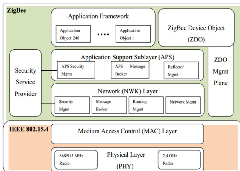
Figure 2. ZigBee protocol stack [8].
