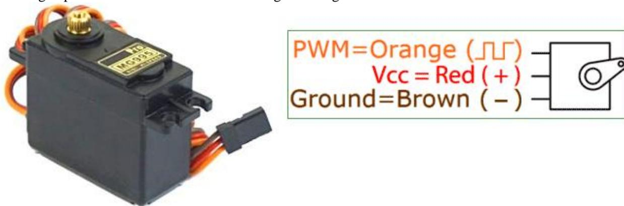
Figure 4. Servomotor
