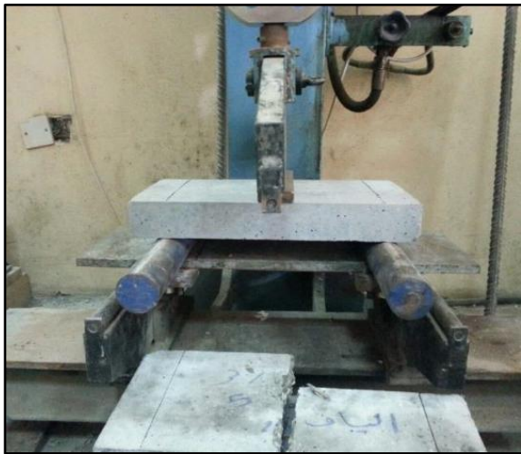
Figure 3. Flexural test of slab
