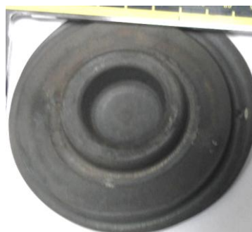
Figure 2. Shape of the forging part after the final forging
