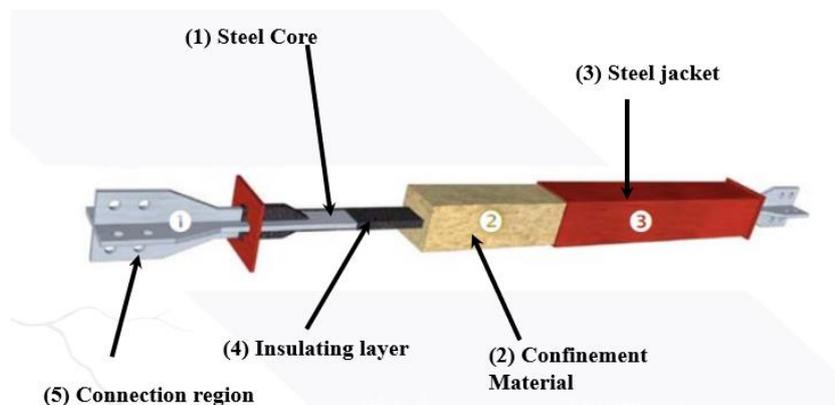
Figure 1. Components of restricted buckling bracing (BRB) according to [21]
