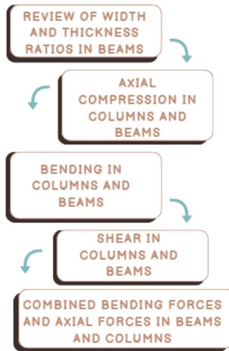
Figure 5. BRB design procedure according to AISC 341
