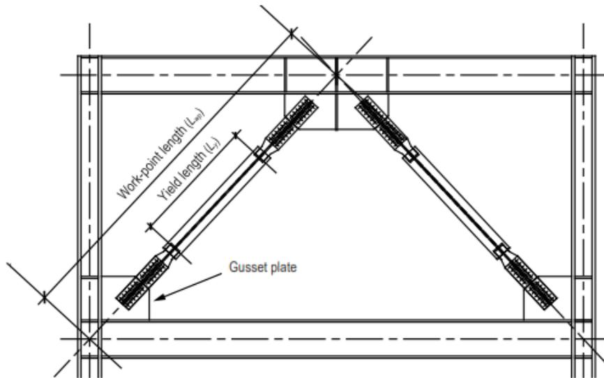
Figure 3. BRB System for X-X Steering: Chevron
