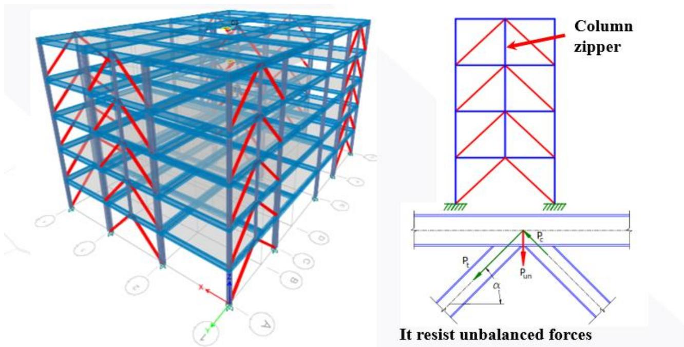
Figure 2. Model of structural steel building
