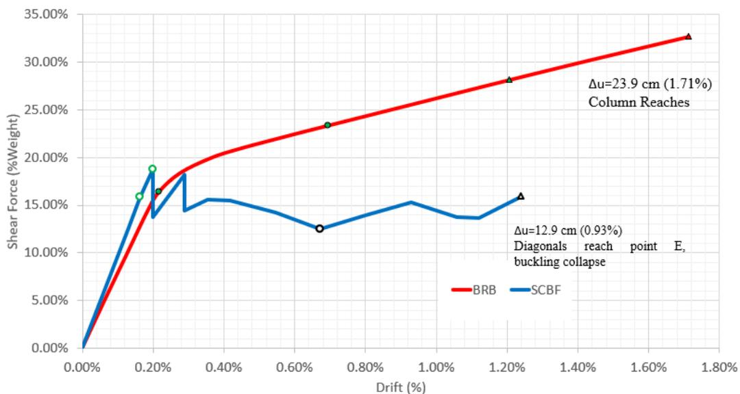
Fig. 10 – Y-Y Direction Capacity Curve
