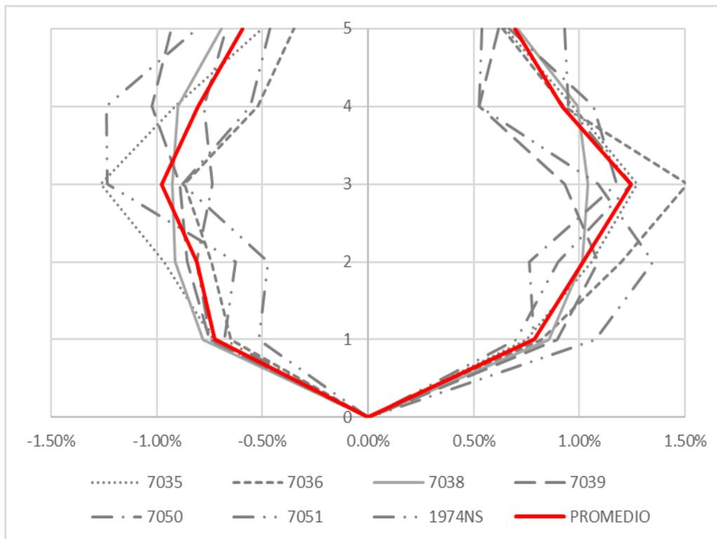
Fig. 14 – DNA mezzanine drifts in the YY direction
