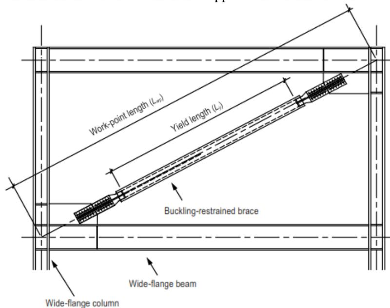
Figure 4. BRB System for Y-Y Direction: Single Diagonal
