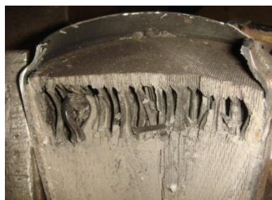
Figure 3. Destruction of the catalytic converter.
