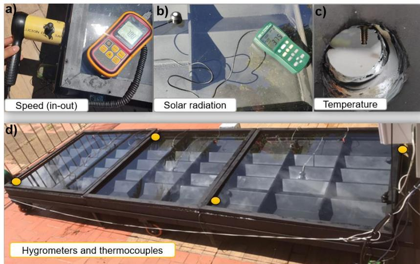
Figure 4. a) Speed meter, b) Solar radiation indicator, c) Temperature indicator and d) Location of thermocouples and humidity sensors
