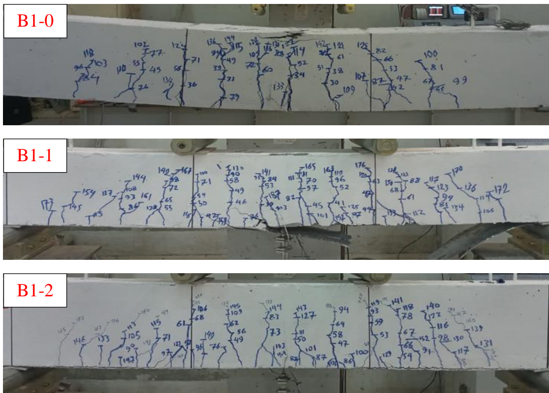
Figure 25. The group (B1) beams, B1-0, B1-1, and B1-2 deformation pattern.
