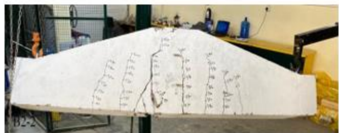
Plate 10. The failure of the (B2-2) beam
