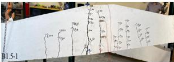
Plate 5. The failure of the (B1.5-1) beam
