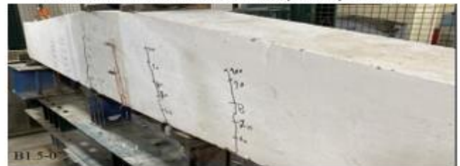
Plate 4. The failure of the (B1.5-0) beam
