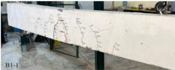
Plate 1. The failure of the (B1-1) beam
