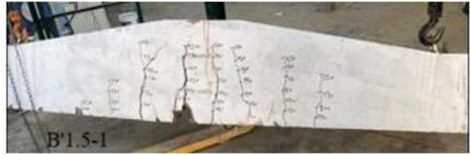
Plate 6. The failure of the (B'1.5-1) beam
