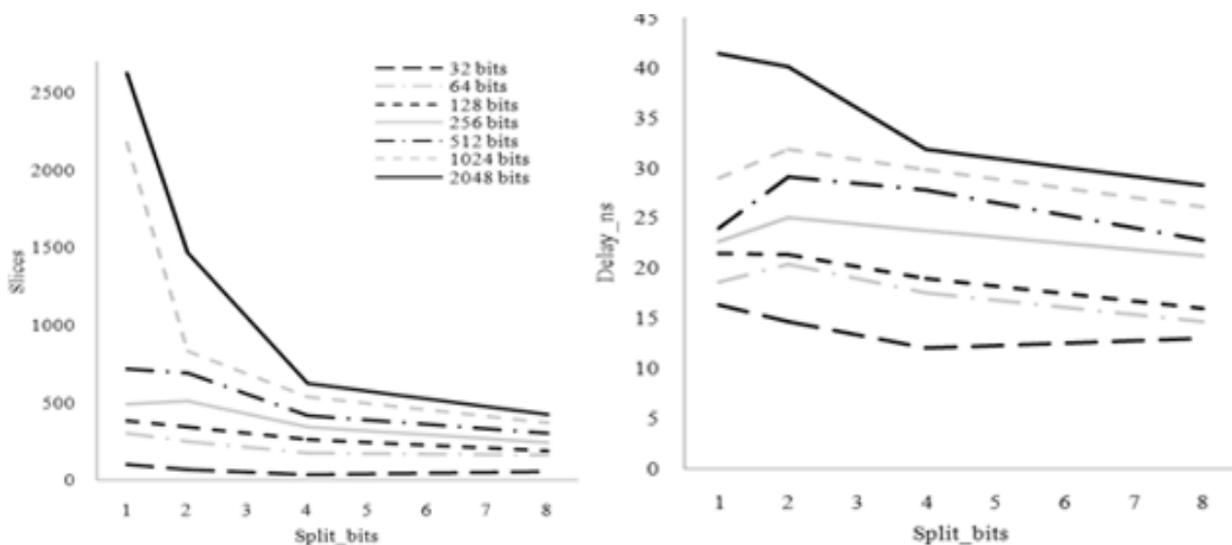
Figure 2. Hardware and time costs for implementing the X mod p operation on a 16-bit FPGA Virtex 6 module, core Xilinx XC6VLX75T a) the number of Slices; b) maximum time delays, ns
