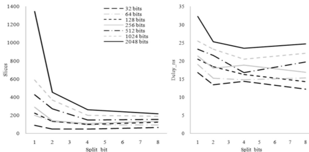
Figure 3. Hardware and time costs for implementing the X mod p operation on an 8-bit FPGA Virtex 6 module, core Xilinx XC6VLX75T a) the number of Slices; b) maximum time delays, ns
