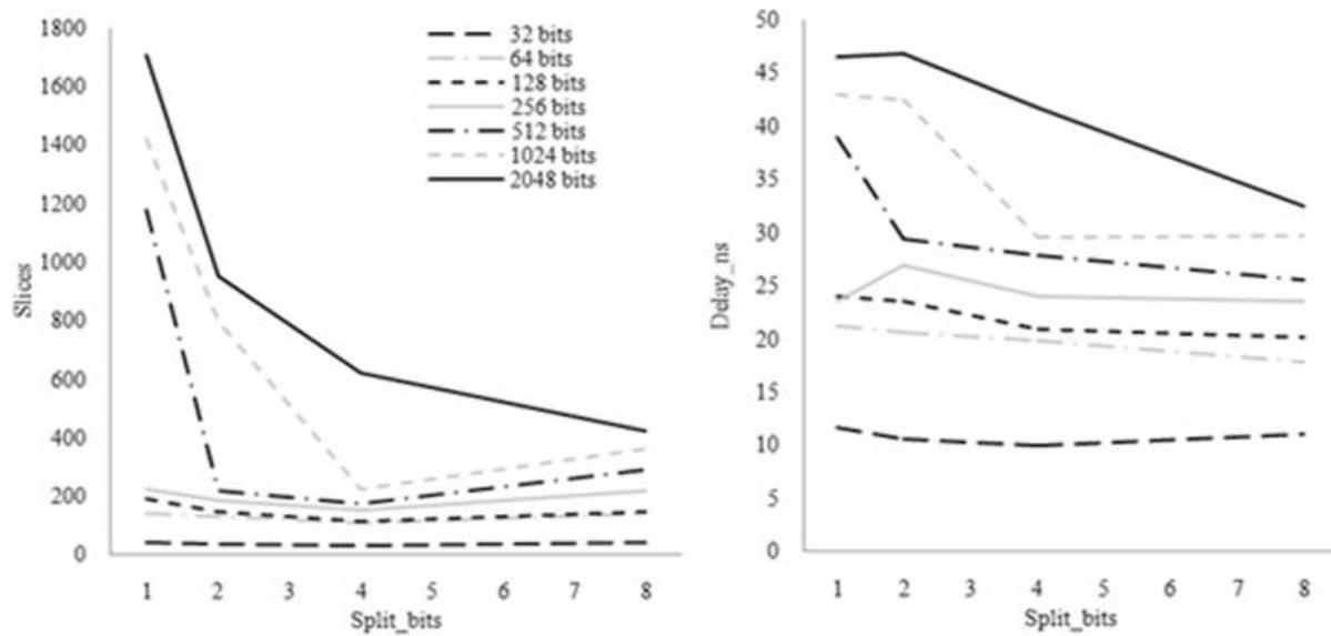
Figure 1. Hardware and time costs for implementing the X mod p operation on a 32-bit FPGA Virtex 6 module, core Xilinx XC6VLX75T a) the number of Slices; b) maximum time delays, ns
