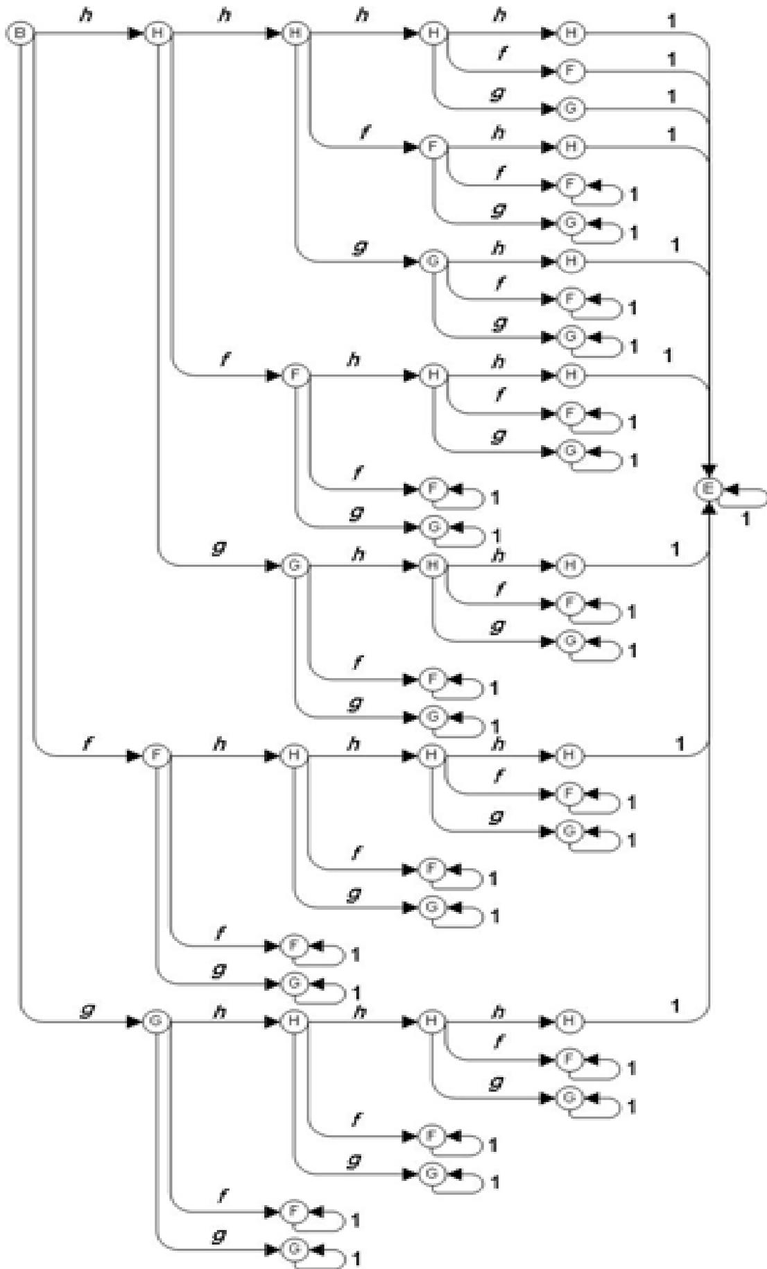
Figure 1. Probabilistic graph of the process of transmitting video streams over the FANET channel
