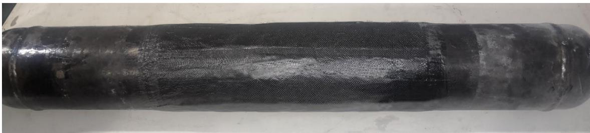
Figure 7. Repaired vessel with carbon epoxy
