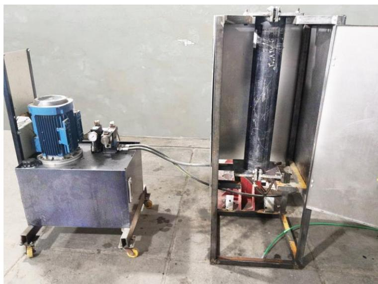
Figure 8. Setup for doing internal pressure tests
