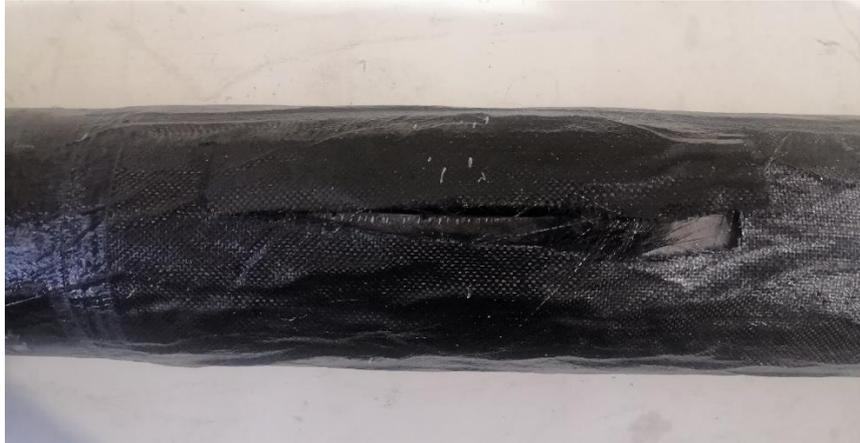
Figure 14. Situation of pipe after burst test
