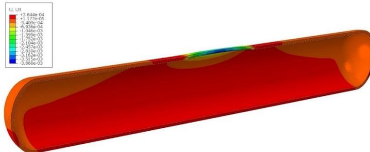
Figure 11. The contour of deformation in the pipe cross-section
