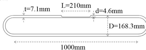
Figure 1. Schematic view of the cracked vessel
