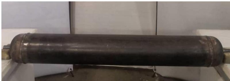
Figure 2. The vessels used for internal pressure tests
