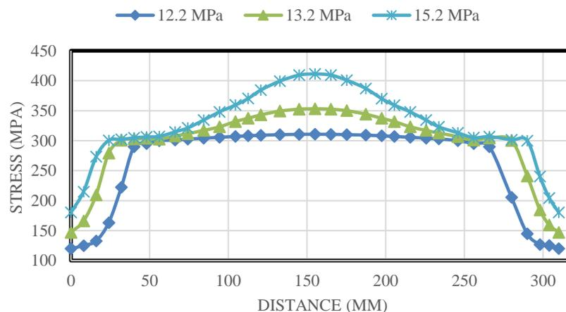
Figure 13. Von Mises stress distribution in pipe.
