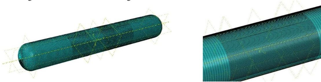
Figure 9. Geometry and mesh configuration of the unrepaired pipe
