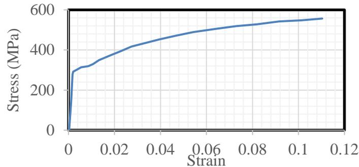
Figure 4. Stress-strain diagram of steel pipes
