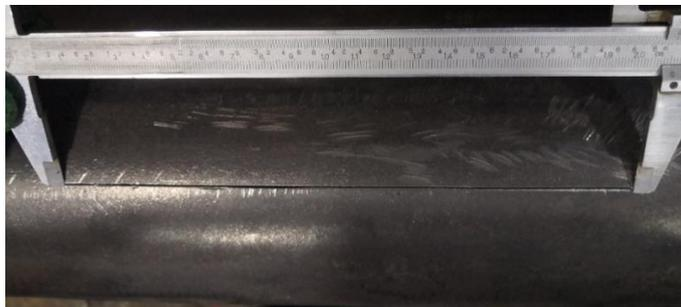
Figure 5. Longitudinal crack with 210mm length and 4.6mm depth considered as defect in central part of the vessel
