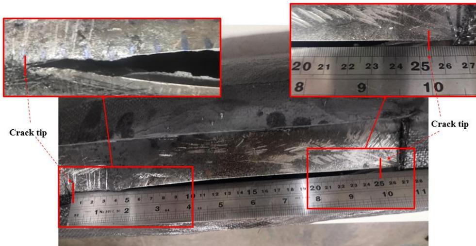
Figure 15. Crack propagation in steel pipe after rupture
