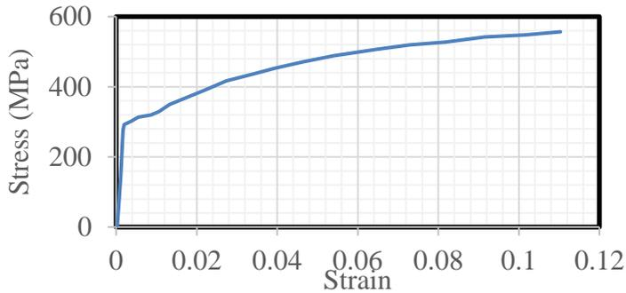
Figure 4. As can be seen in this figure, yield and ultimate stresses of the pipes is 300MPa.
