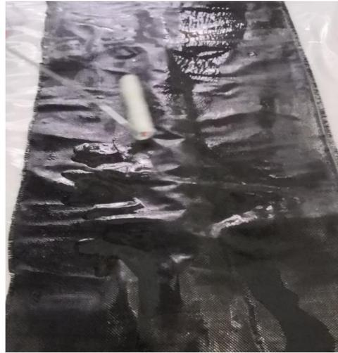
Figure 6. Saturation of carbon fabric with epoxy resin
