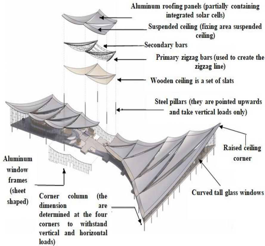
Figure 4. Shows the details of the structural system and components of Vastetas Travel Center [25]
