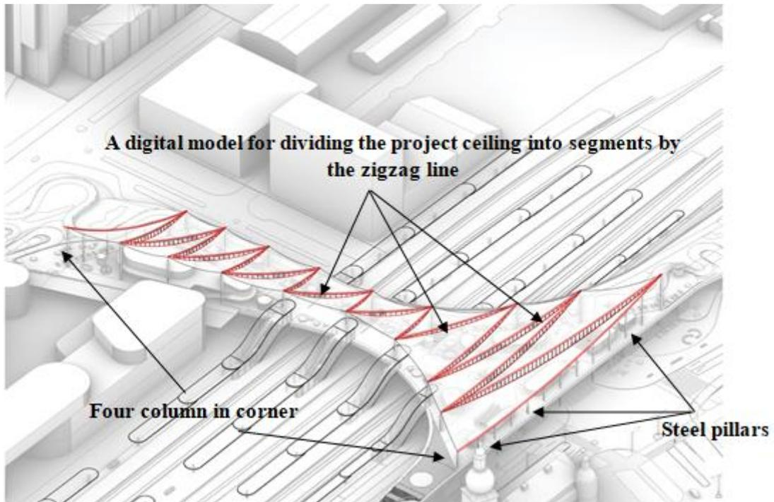
Figure 3. Shows the digital model of Vastetas Travel Center [25]
