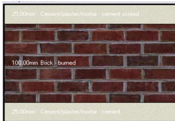
Figure 2. Composition of the layers of the outer wall
