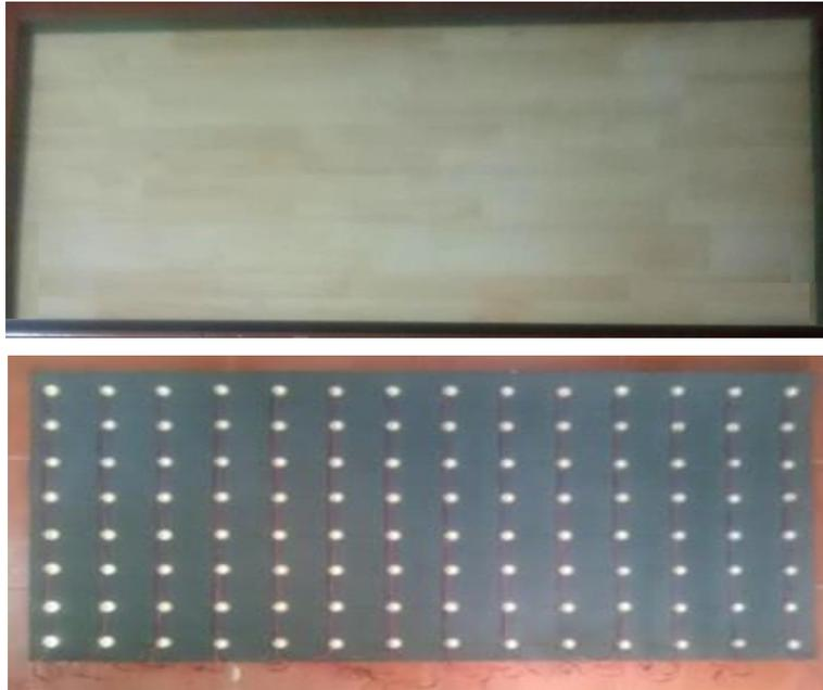
Figure 5. Top and bottom view of the piezoelectric tile constructed
