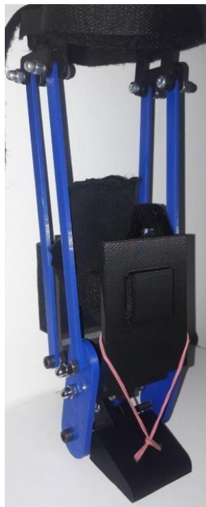
Figure 13. Printed prosthesis with its component elements such as Velcro, elastic, screws and nuts
