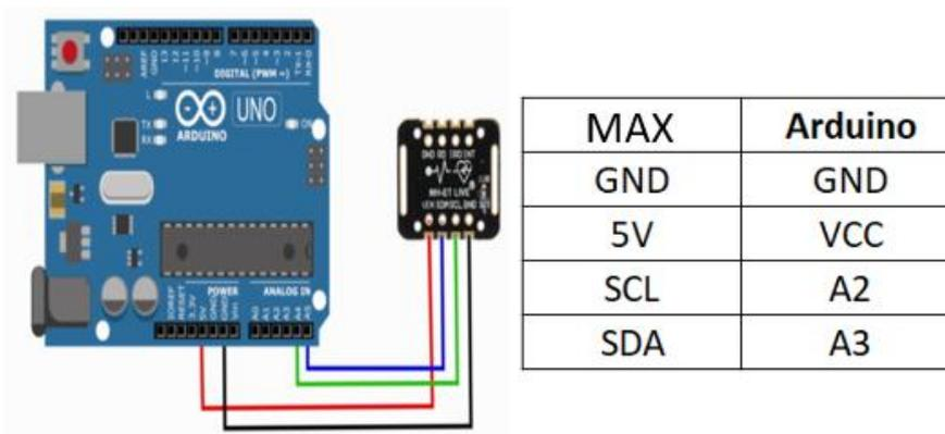
Figure 6. Connection between Arduino and MAX 30102 Sensor
