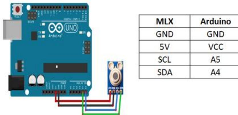
Figure 5. Connection between Arduino and MLX 90614 Sensor
