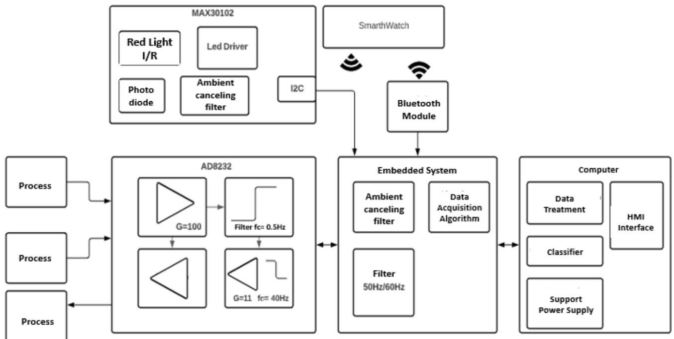
Figure 3. Embedded System Block Diagram.
