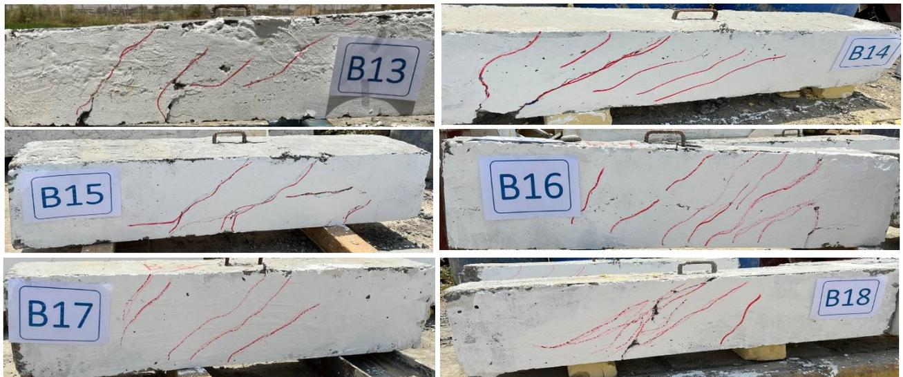
Figure 9. Crack pattern for group 2
