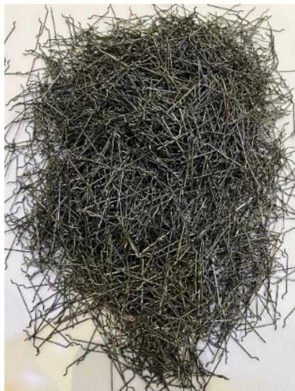
Figure 2. Hooked steel fibers
