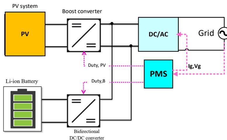
Figure 3. Proposed PV-battery grid connected inverter
