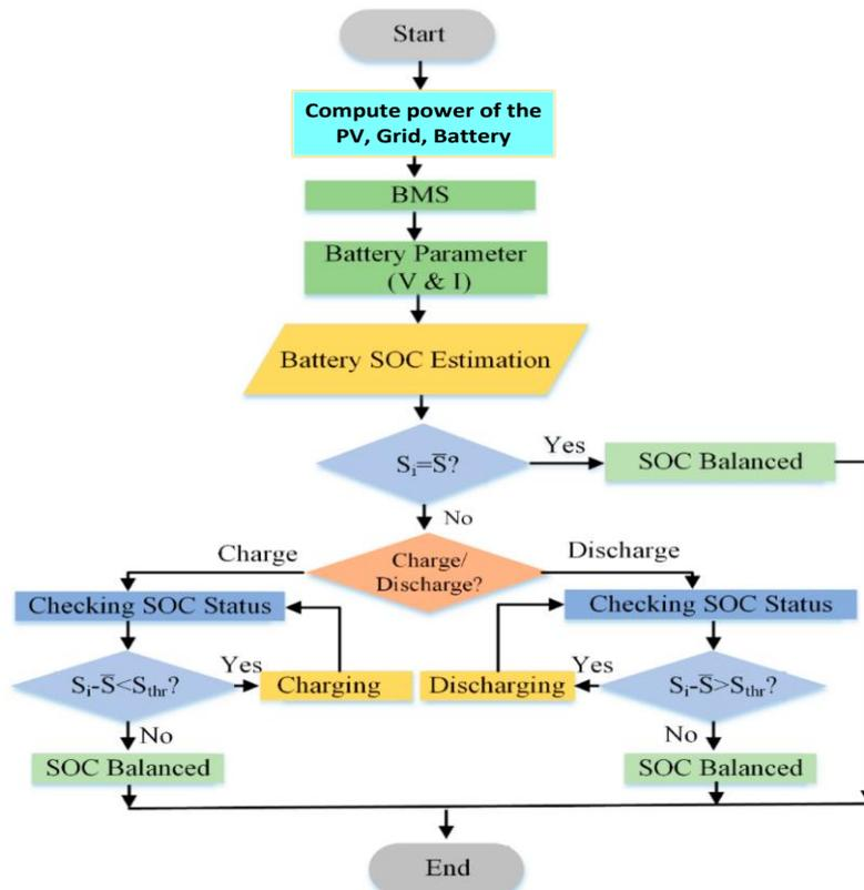
Figure 7. It proposed PMS algorithm of the hybrid PV-battery inverter
