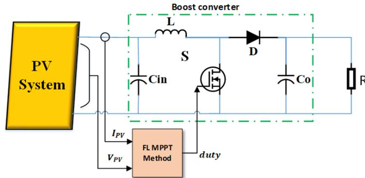
Figure 6. FL MPPT controller with boost converter circuit
