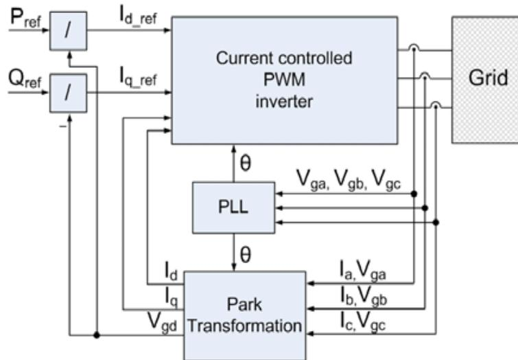
Figure 8. PQ control method for VSC inverter
