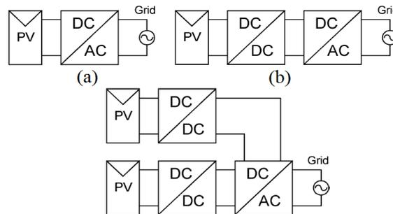
Figure 1. PV inverter architectures-based power stage unit (a) single stage inverter (b) two stage inverter (c) Multi stage inverter
