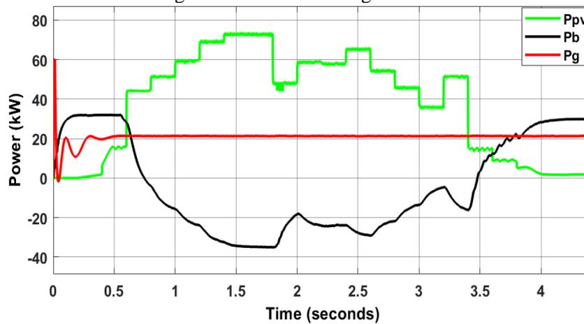
Figure 13. Power curves of the battery, PV and grid at varied solar irradiation case
