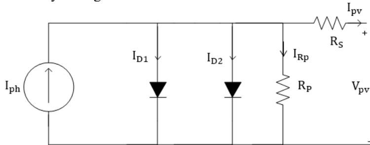
Figure 3. Two-diode PV cell model
