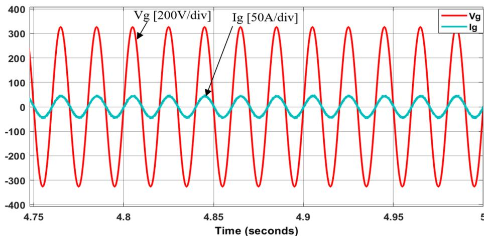
Figure 16. The results of the injected current to the grid with grid voltage
