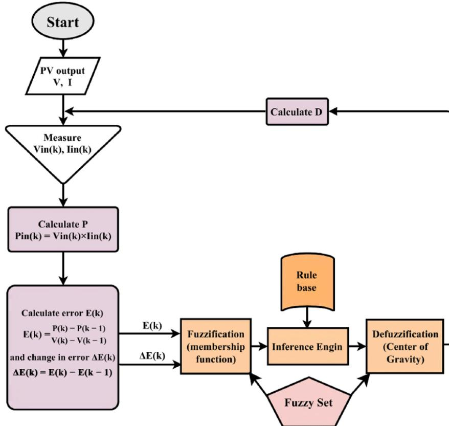
Figure 4. The FL algorithm based MPPT
