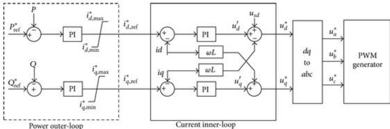
Figure 9. detailed model control of the PQ technique
