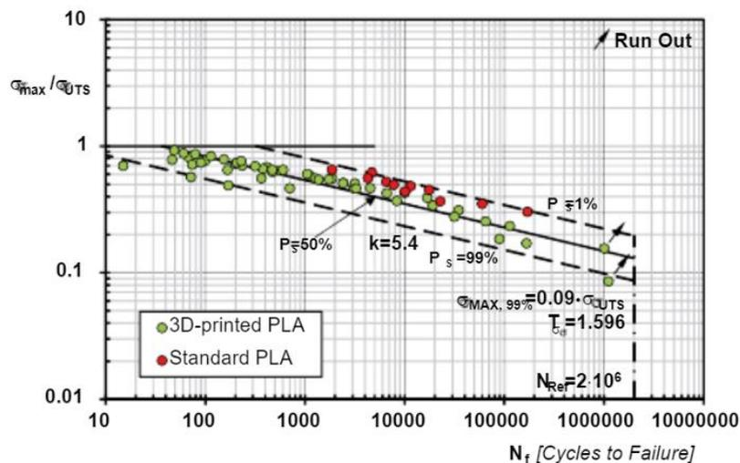
Figure 5. Fatigue strength of standard PLA vs. fatigue strength of AM PLA
