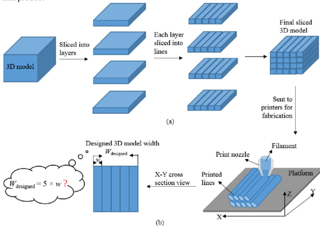
Figure 1. Main process stages common to most RP systems
