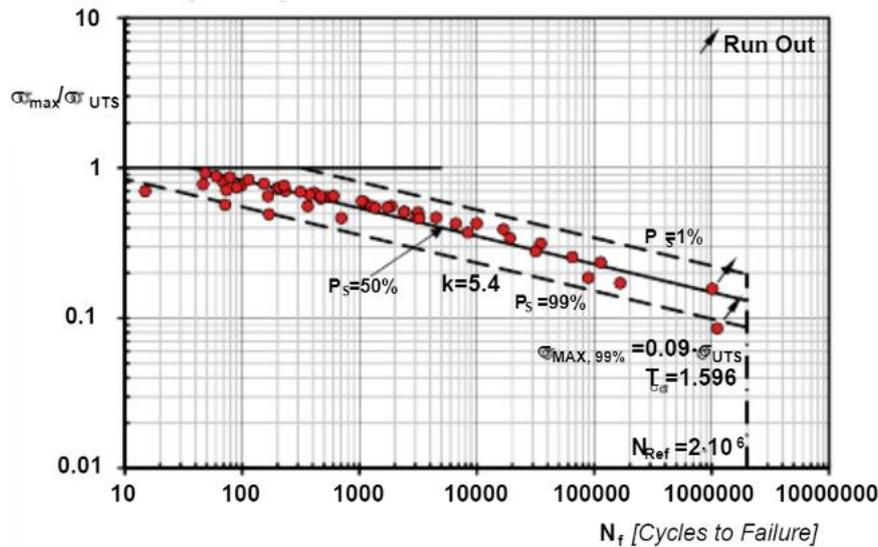
Figure 4. Design fatigue curves normalized (for an infill level equivalent to 100 percent)
