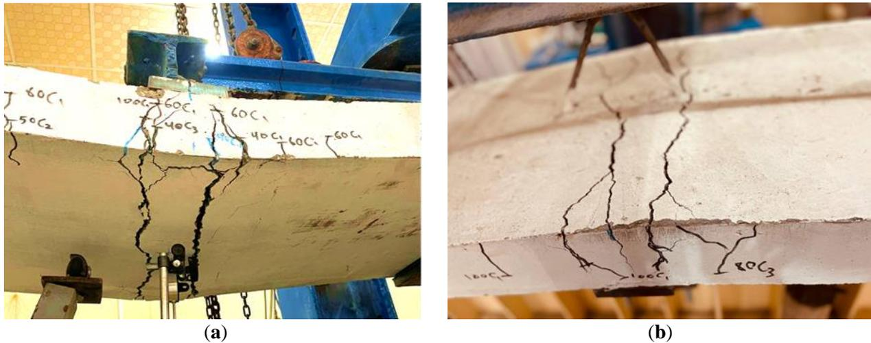
Figure 9. Photos of the control S9 specimen at failure: (a) Failure of mid-span section (sagging region); (b) Failure of section over central support (hogging region)
