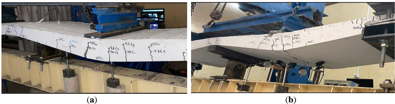
Figure 10. Typical Cracks pattern at failure for slabs of this study: (a) Cracks pattern for non-prismatic simply supported slab with positive haunch (S2 specimen); (b) Cracks pattern for non-prismatic fixed end support slab with positive haunch (S5 specimen)
