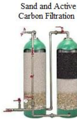
Figure 8. Sand and active carbon filtration Source: Author's elaboration
