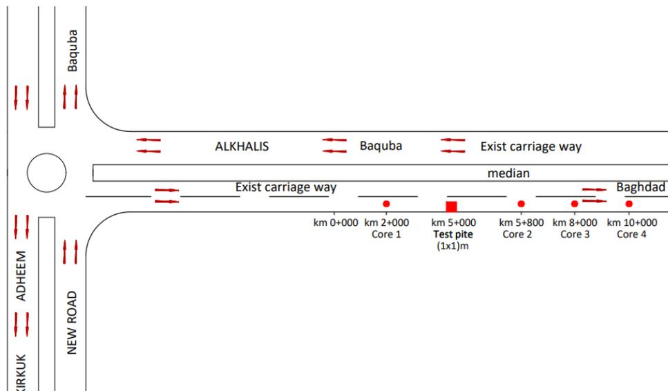
Figure 2. The locations of the samples extracted from field in the study area
