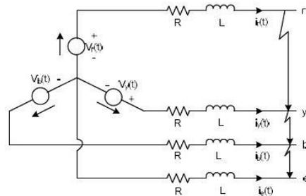
Figure 1. Basic balanced three-phase electric circuit with earth return
