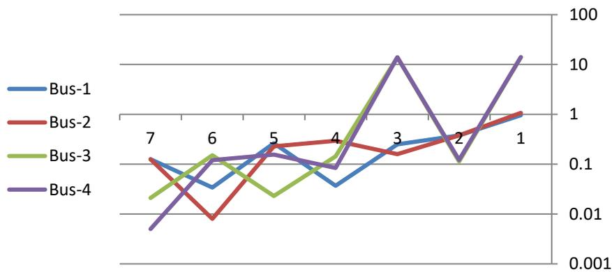
Figure 4. Distribution of fault currents in four different buses on Qadsiya substation
