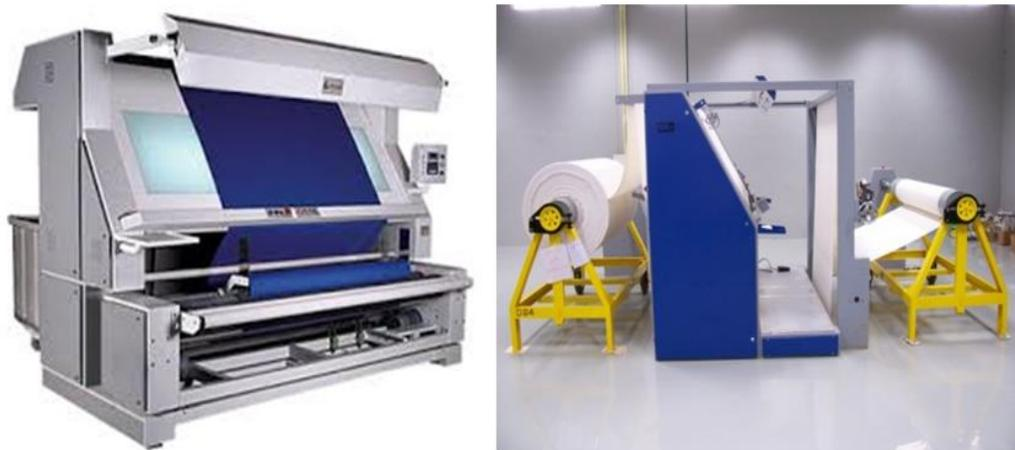
Figure 1. Fabric inspection machine
