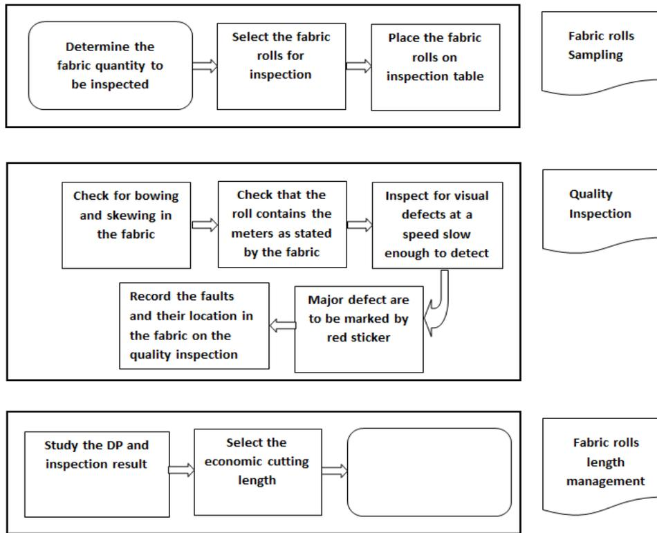
Figure 2. Fabric rolls inspection procedure
