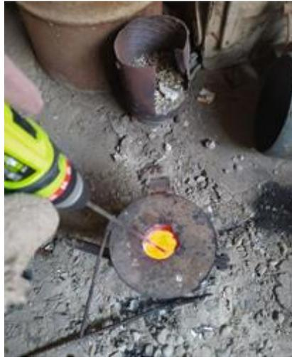
Figure 3. Stir casting process
