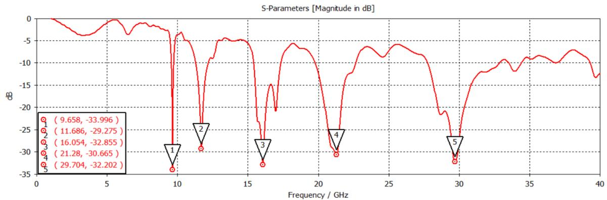
Figure 3. The reflection coefficient ( $S_{11}$ ) versus frequency
