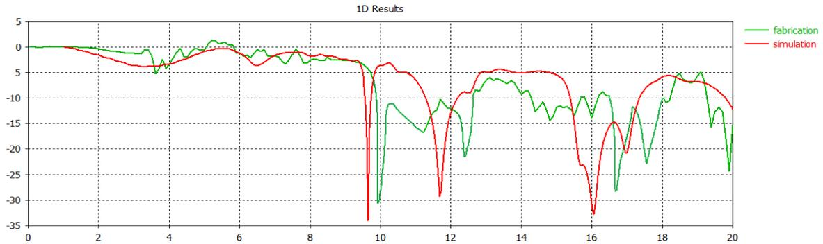
Figure 7. The shows the reflection coefficient ( $S_{11}$ ) versus frequency of simulation and fabrication results
