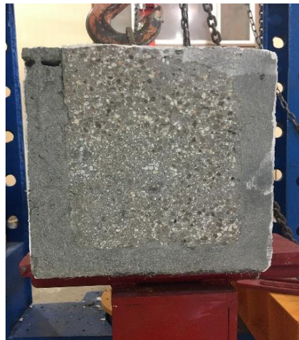
Figure 8. SIFCON jacket cover three faces of beam specimen
