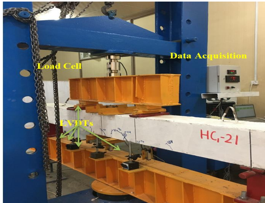
Figure 9. LVDTs and Load Cell Installed on the test machine
