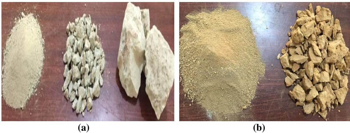
Figure 2. Montmorillonite clays, (a) before burning, (b) after burning
