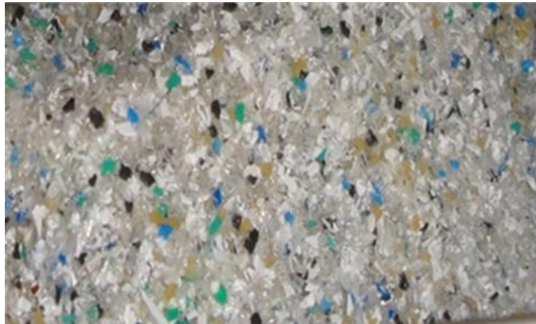
Figure 1. Shredded BMW: mixing of small pieces of shredded components rapidly contaminate the entire pile of waste
