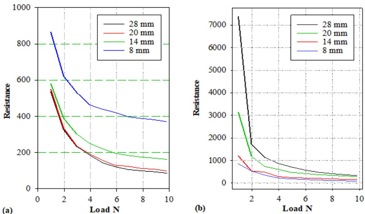
Figure 8. (a) The resistance of single output sensor during static load test for four different diameter of compression disc. (b) The resistance of matrix sensor during static load test for four different diameter of compression disc
