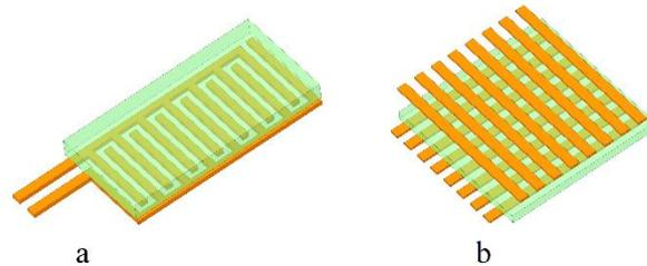
Figure 1. Sensor design. (a) Single output sensor design. (b) multioutput matrix sensor design
