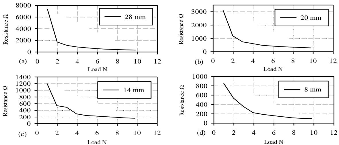
Figure 5. The resistance reading of multioutput matrix sensor design during static load test for four different diameter of compression disc. (a) compression disc with diameter = 28 mm. (b) compression disc with diameter = 20 mm. (c) compression disc with diameter equal 14 mm. (a) compression disc with diameter = 8 mm
