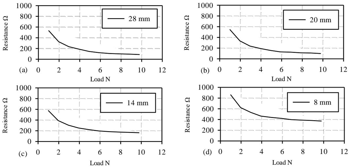
Figure 4. The resistance reading of single output sensor design during static load test for four different diameter of compression disc. (a) compression disc with diameter = 28 mm. (b) compression disc with = equal 20 mm. (c) compression disc with diameter = 14 mm. (a) compression disc with diameter = 8 mm
