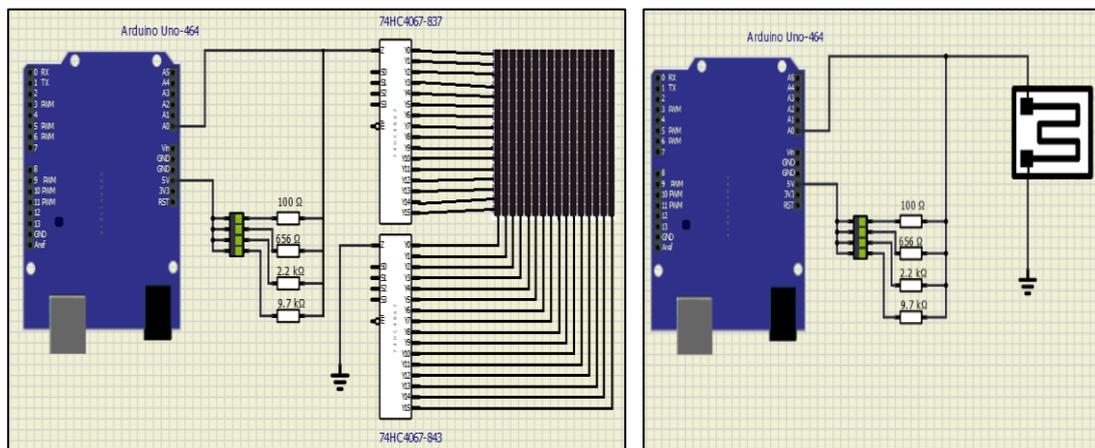
Figure 3. Schematic diagram for resistance measurement circuit. (a) Measurement circuit for the multioutput matrix sensor. (b) Measurement circuit for the single output sensor design
