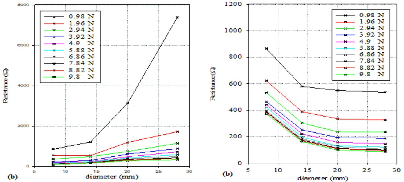
Figure 9. (a) Effect of the contact area on the resistance reading of single output sensor design. (b) Effect of the contact area on the resistance reading of matrix sensor design
