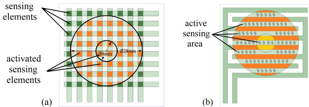
Figure 10. (a) applying two different compression disc size on the single output sensor. (b) Applying two different compression disc size on the multioutput matrix sensor.
