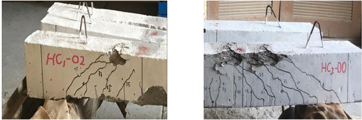
Figure 17. Failure of beam without strengthening of SIFCON jacket
