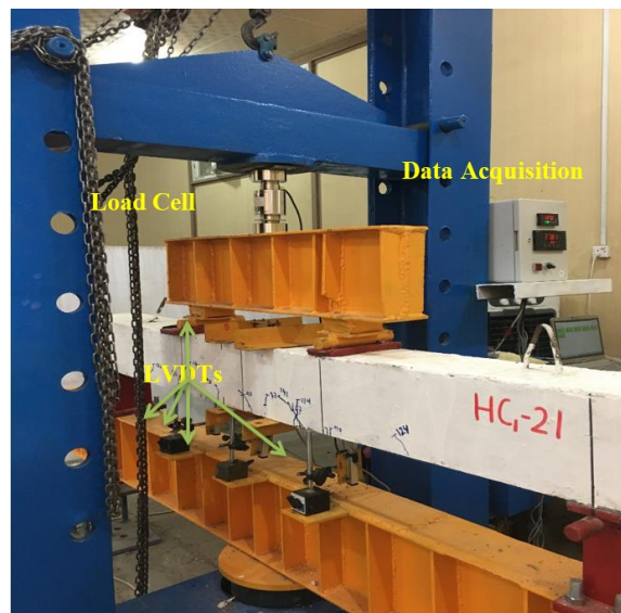
Figure 10. Arrangement of LVDTs and Load Cell within the test device
