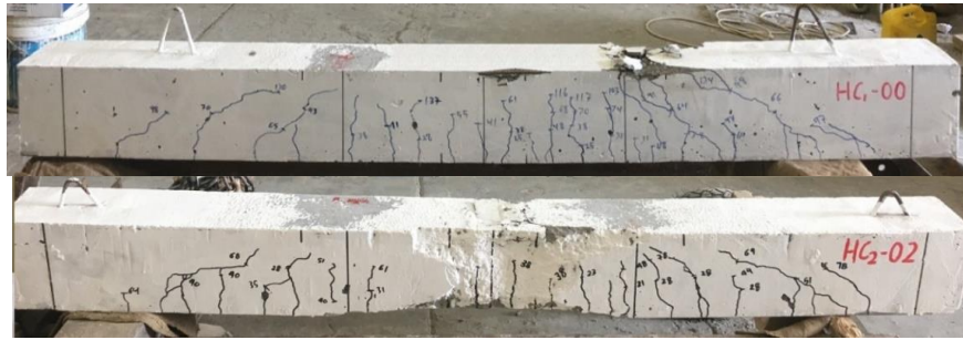
Figure 13. Cracks pattern of HSC LWC beams before and after burning
