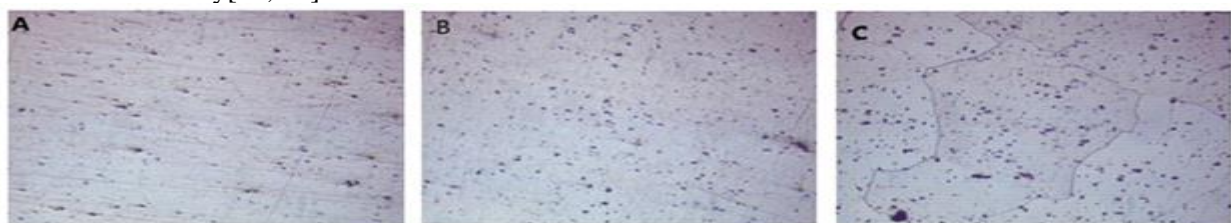
Figure 1. microstructure of Al 6061 after aging for: (A) 30 min (B) 120 min (C) 240 min. At 400 X
