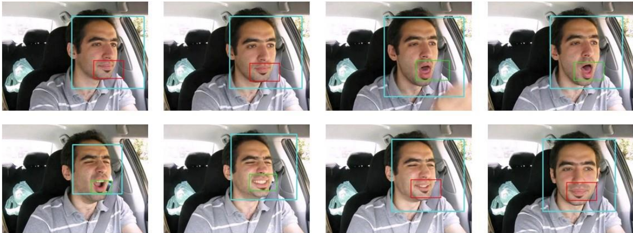
Figure 12. The classification of tiredness and fatigue on human faces by tracking the face expression where green rectangular region predicts the driver tiredness as well as fatigue however the red rectangular on face predicts the driver alertness
