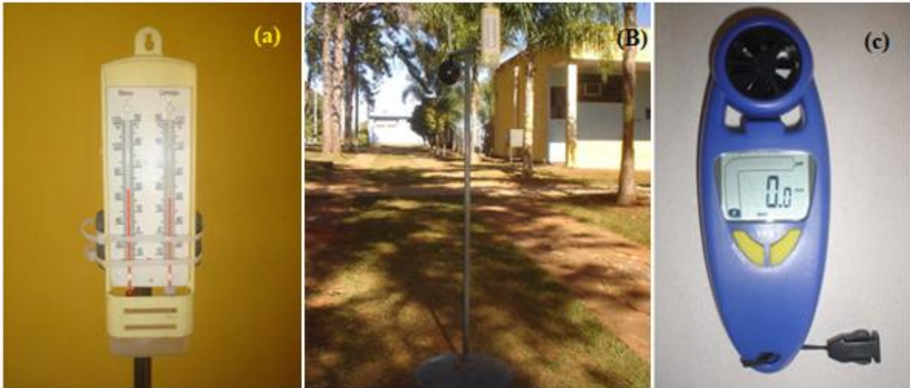
Figure 3. (a) Natural ventilation psychrometer. Detail of the equipment height at 1.30 m, (b) Set of thermometers composed of the natural ventilation psychrometer and the dry bulb thermometer inserted in the black globe. (c) Portable digital anemometer
