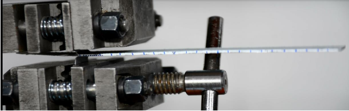
Figure 7. T-peel specimen on universal testing machine
