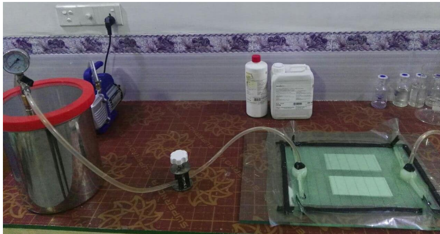
Figure 5. VARTM fabrication process
