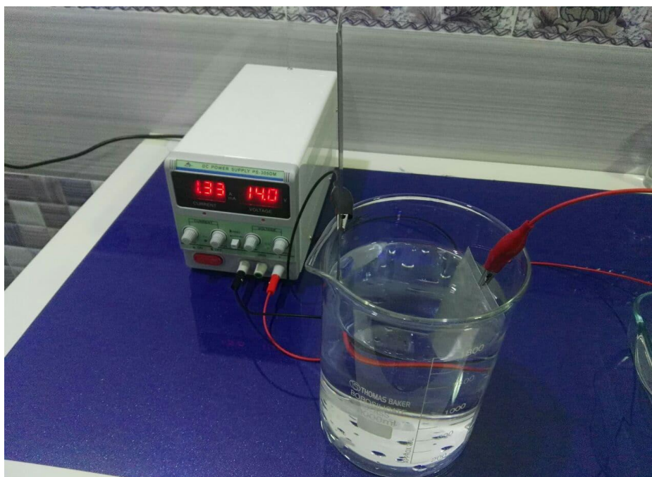
Figure 1. Anodization cell with electrolytic bath
