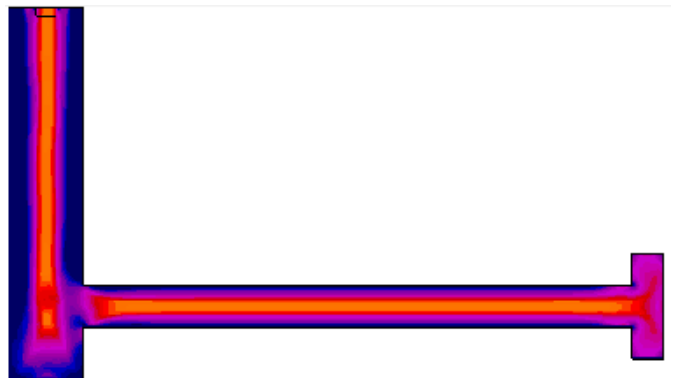
(f) Permanent mould (120°C), cast at 750°C
