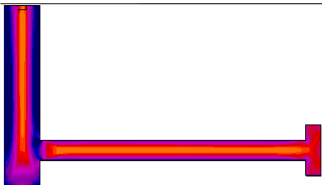
(g) Permanent mould (250°C), cast at 700°C
